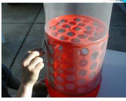
Next: Remove the two small pieces of Duct Tape on the outside. Run a bead around the measuring lip at the top, and a bead around the very bottom of the bucket. Pull your screen around the bucket and over-lap the first joint. Tape the screen to itself to hold in place. Now, run
