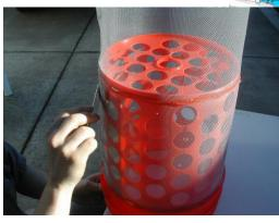
Next: Remove the two small pieces of Duct Tape on the outside. Run a bead around the measuring lip at the top, and a bead around the very bottom of the bucket. Pull your screen around the bucket and over-lap the first joint. Tape the screen to itself to hold in place. Now, run
