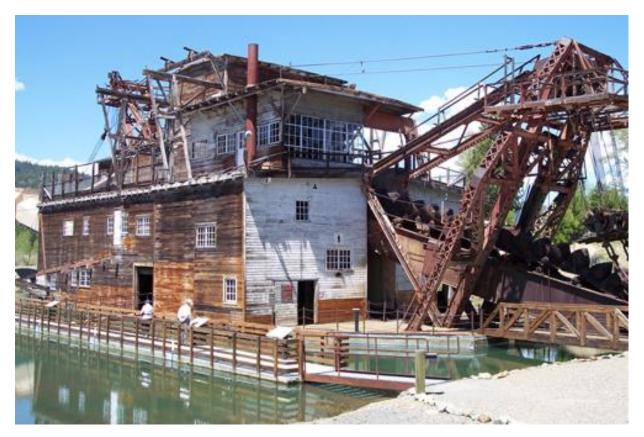
This is Dredge No.3, The last one made and is still in Sumpter Oregon. It is stuck in its own little pond made by the buckets as it dug along collecting dirt and rocks and YES!!! GOLD, a lot of it.
