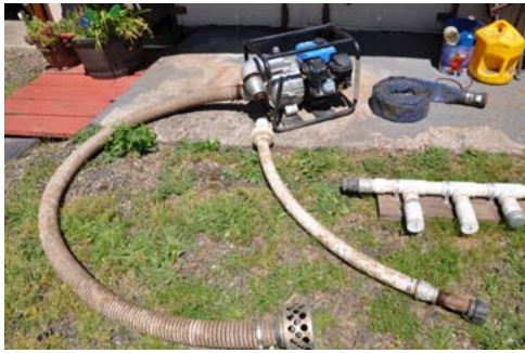
3" water pump with manifold for additional outputs
