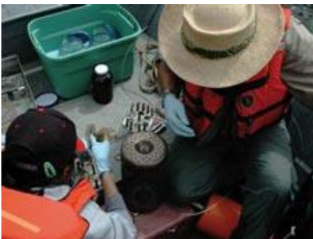
OSU researchers designed sampling equipment that would absorb dissolved chemicals from the river water just like a fish or human would. Photo: Kim Anderson
